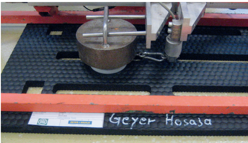
Figure 5: Slip resistance measurement
